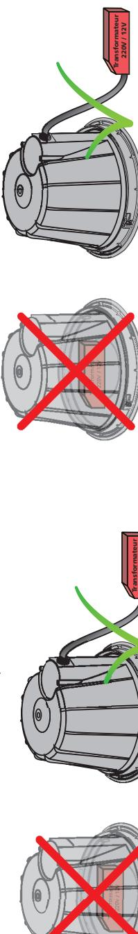
Compatibility between types of bulb and insulation (in roll or loose):
